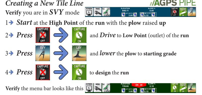
5 Toggle Machine Control on your tractor and lay the run
