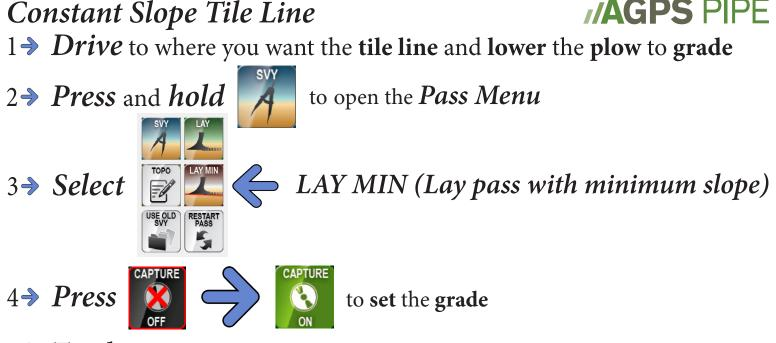
5 Toggle Machine Control on your tractor and lay the tile
